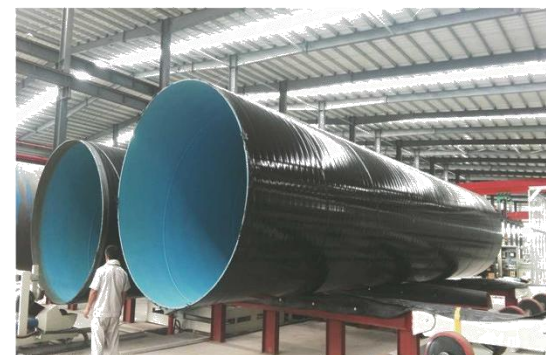
φ 800-φ 2800钢管内壁环氧粉末、外壁三层PE生产线 (TPEP) φ 800-φ 2800 pipe internal wall epoxy powder, external wall three layer PE production line (TPEP)
