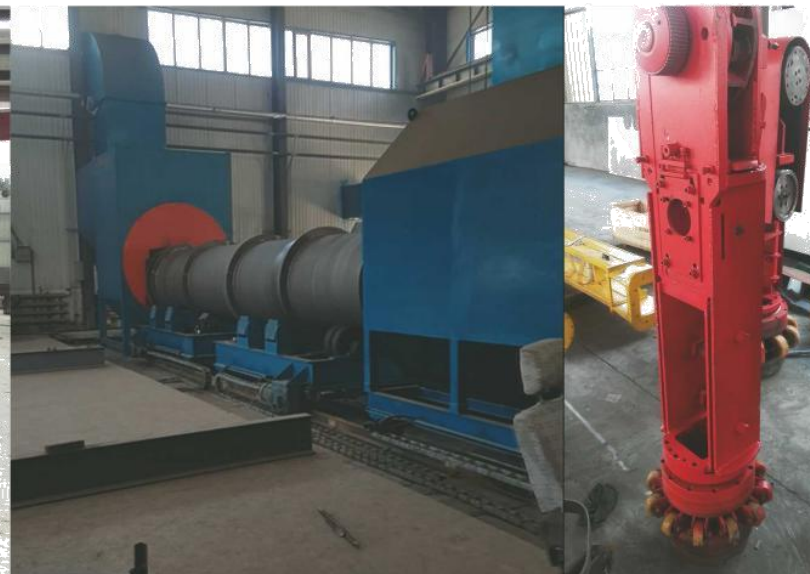
φ 1000-φ 2800带加强筋法兰特殊钢管内壁除锈生产线 φ 1000-φ 2800 with reinforced flange special steel pipe inner wall rust removal line
