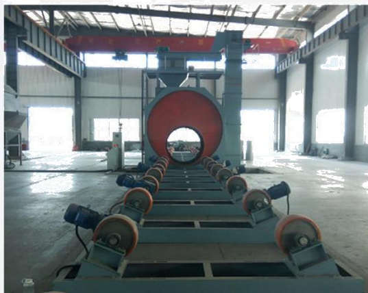
φ 3500 外壁抛丸除锈生产线 φ 3500 outer wall shot blasting and rust removal line
