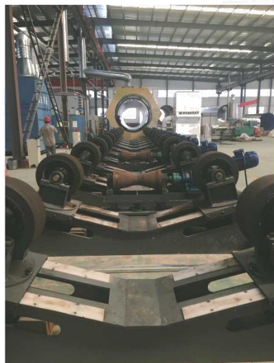
钢管大口径单组螺旋输送线 Large diameter single spiral conveying line for steel pipe
