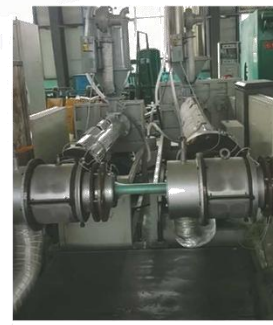
钢管包覆3PE生产线 (φ 32 - φ 325) Steel pipe coated 3 PE production line (φ 32 - φ 325)
