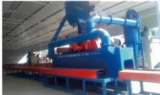
钢管外壁多管抛丸除锈机 Multi-pipe shot blasting and rust removal machine for outer wall of steel pipe
