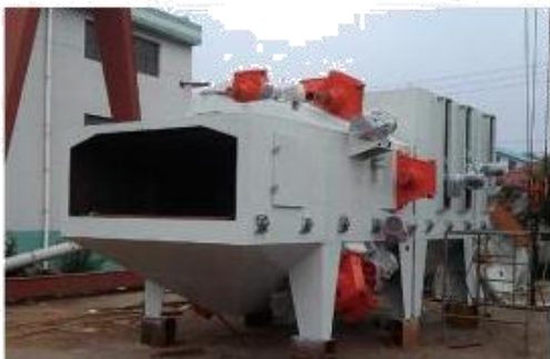
钢管、钢板、型材综合式多功能抛丸除锈机 Steel pipe, steel plate, profile comprehensive multi-functional shot blasting and rust removal machine
