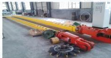
钢管内壁抛丸除锈、抛头枪杆扶正器 Shot blasting and rust removal on inner wall of steel tube, gun centralizer
