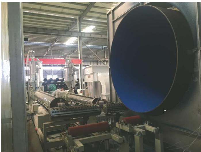
φ 800-φ 3200钢管内壁环氧粉末、外壁三层PE生产线 (TPEP) 800-3200 the outer wall of steel pipe wall epoxy powder, three layer PE production line (TPEP)
