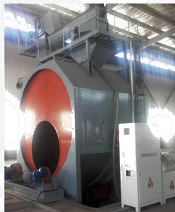
φ 3500 外壁抛丸除锈生产线 φ 3500 outer wall shot blasting and rust removal line
