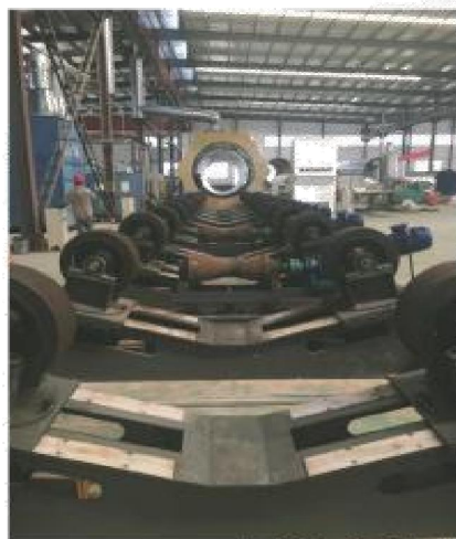
钢管大口徑单组螺旋输送线 Large diameter single spiral conveying line for steel pipe
