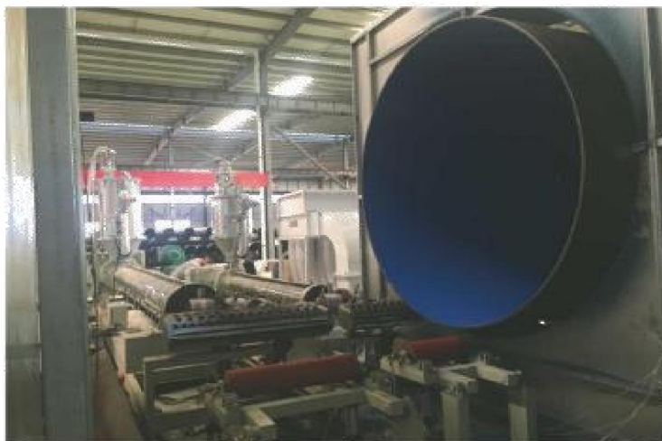
φ 800-φ 3200 钢管内壁环氧粉末、外壁三层PE生产线 (TPEP) 800-3200 the outer wall of steel pipe wall epoxy powder, three layer PE production line (TPEP)
