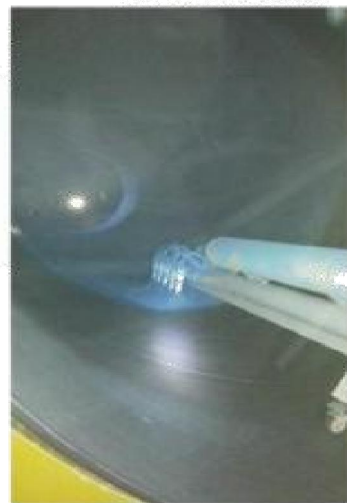
内壁粉末喷涂 Powder Spraying on Inner Wall
