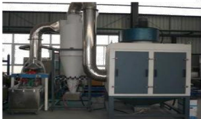
环氧粉末回收系统 Epoxy powder recovery system
