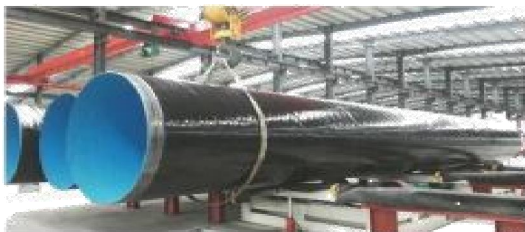
Large diameter TPEP finished pipe
