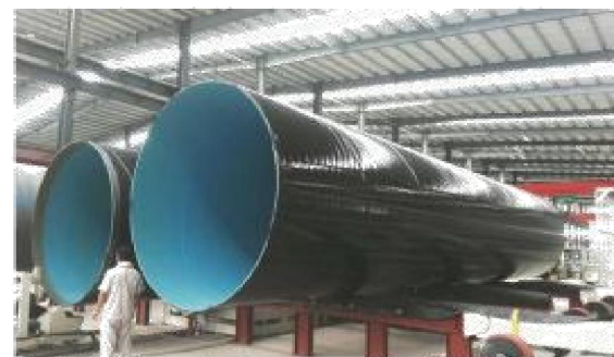
φ 800-φ 2800 钢管内壁环氧粉末、外壁三层PE生产线 (TPEP) φ 800-φ 2800 pipe internal wall epoxy powder, external wall three layer PE production line (TPEP)
