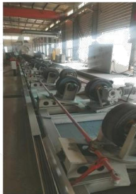
φ 159-φ 1020 钢管3PE防腐生产线 φ 159-φ 1020 pipe 3PE anticorrosive production line
